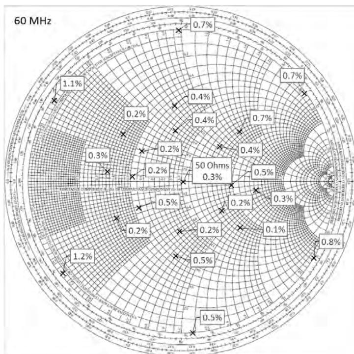
Figure 5: Typical 60 MHz impedance verification against VNA.
