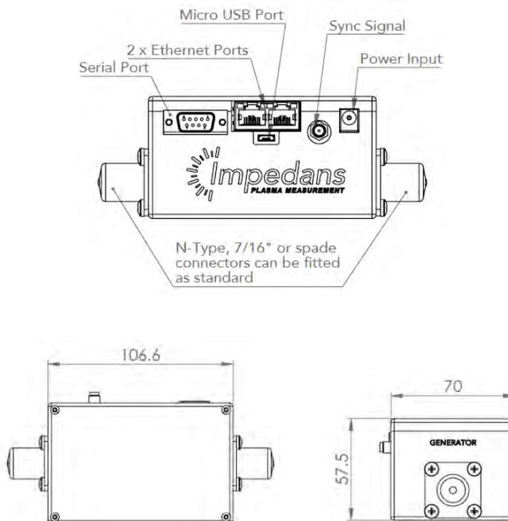
Figure 1: Dimensional drawings of the standard Octiv Poly model 02-232-01 with Quick Change RF connector interface. All dimensions are in mm. Contact Impedans for dimensional drawings of other models.
