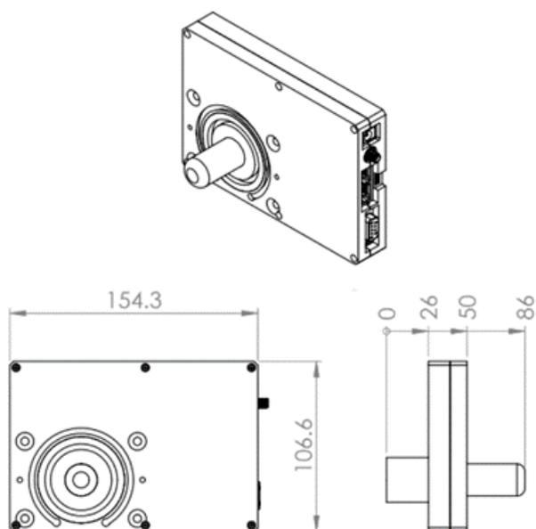
Figure 2: Dimensional drawings of model 02-0308-01.
